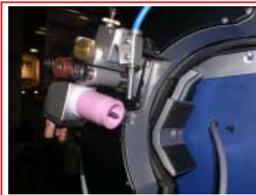
ORBIWELD TP Head with AVC & Oscillation
