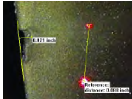
Highly accurate laser measurement can be used as a Go/No Go comparator
